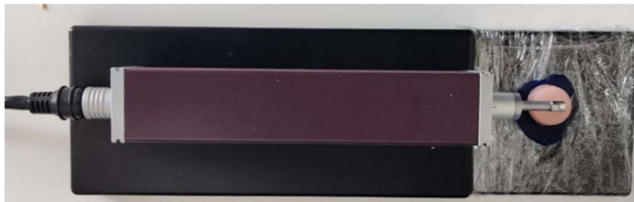
Figure 4: MEASURING SURFACE ROUGHNESS OF SAMPLE USING STYLUS - 2µm/60
