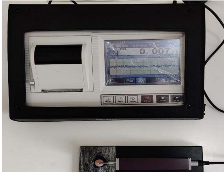
Figure 2: MITUTOYO SJ-310 Stylus Profilometer
